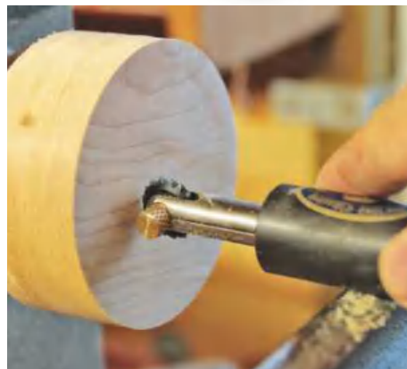
▲ A flat on the sleeve sits on the toolrest, which delivers support and retains the correct angle
